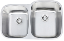
CRESCENT STAINLESS STEEL SINK 60/40 REVERSE DOUBLE BOWL 18G INSTALLATION: UNDERMOUNT EXTERIOR DIMENSIONS: 32-1/4" X 20-5/8" X 9"-7" TR4060-18
